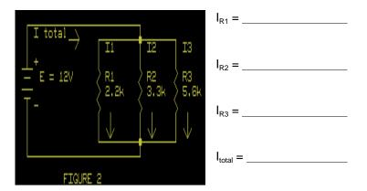
3. Add the measured currents through R<sub>1</sub>, R<sub>2</sub>, and R<sub>3</sub> together and compare with the measured total current. Record the sum of measured currents.
