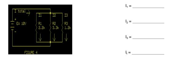
3. Change the value of  $R_2$  to 5.6 k $\Omega$ . Again measure the current through each resistor, and the total current, and record below.
